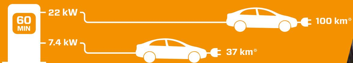
\* EV cable 22 kW: 1-hour charging up to 100km EV range, depending on EV model and charger.
